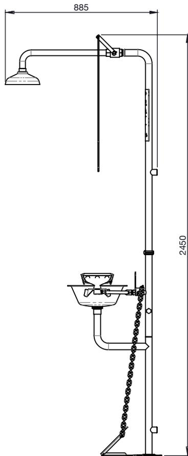
**Inlet and Outlet Connections: 25mm BSPM**
